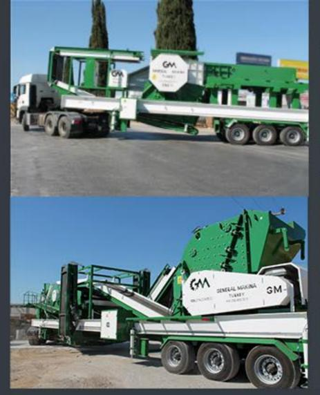
GNR - MC110 Mobile Jaw Crusher plant includes a 110 mobile jaw crusher group with mobile feeder independently operating. In addition to a mobile impact crusher (DMK 03), and mobile vibrating screen.
